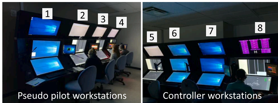
Fig. 11. The Phoenix TRACON simulator (eight operational workstations) for pseudo pilots and controllers.
