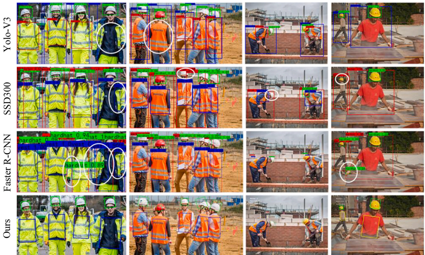
Fig. 18. Qualitative comparisons with state-of-the-art methods. Examples annotated with white ovals correspond to false detections.
