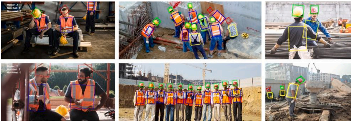
Fig. 17. Qualitative results of the proposed method. Different object categories are labeled in different colors. Red color – non-hardhat use; Green color – hardhat use; Yellow color – non-vest use; Blue color – vest use. (For interpretation of the references to color in this figure legend, the reader is referred to the web version of this article.)
