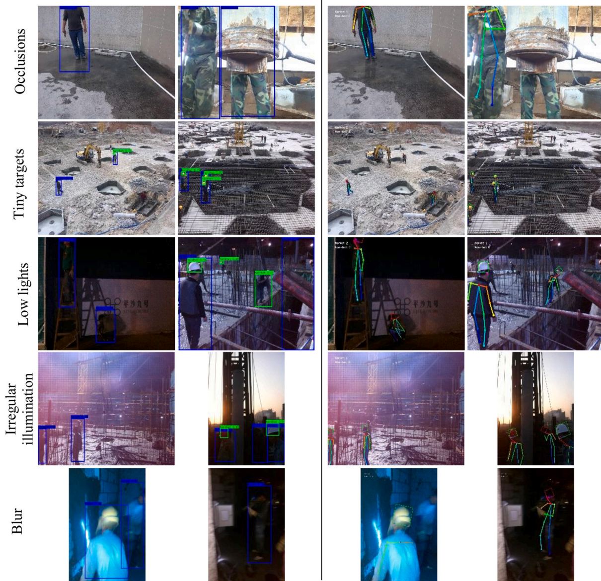
Fig. 19. Qualitative comparisons with state-of-the-art methods in challenging scenarios. Left: YOLO-v3 model; Right: The proposed method.
